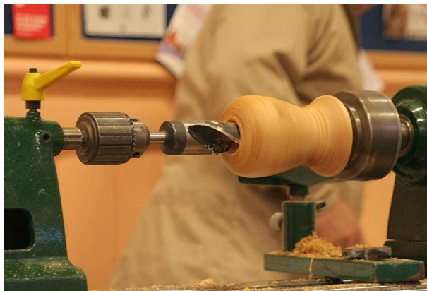
boring the centre out
