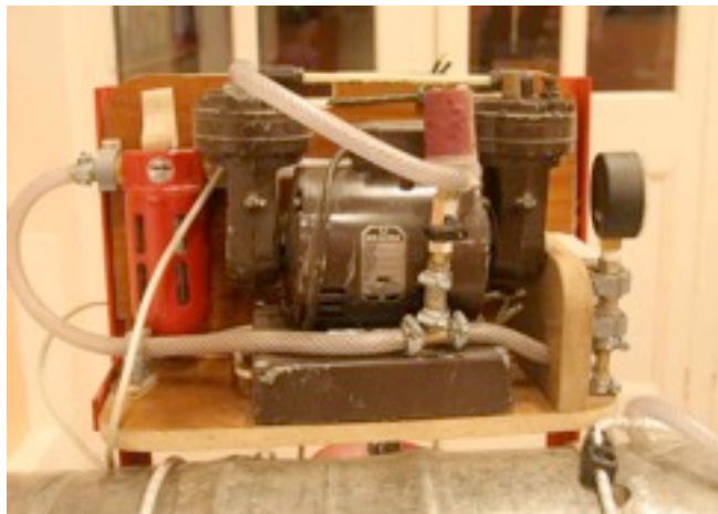
The motor, pump arrangement
